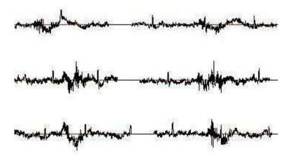
Figure 6.2: EMG signals for the words no (first), accept (middle) and yes (last) and speaker S1 (EMG1, session 008)
