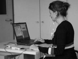
Figure 4.1: Physiological data recording system (Amplifier of the VARIOPORT\_VIII system (left), recorder (middle), and electrical isolater (right)) and setup for data recording session
