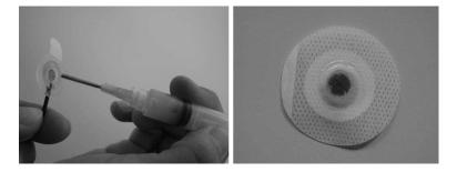
Figure 4.2: Reusable detection electrode filled with gel (left) and disposable ground electrode (right).
