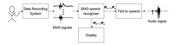
Figure 7.1: Schematic view of silent phone prototype
