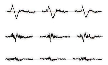
Figure 6.1: EMG signals for the words no (first), accept (middle) and yes (last) and speaker S0 (EMG1, session 008).
