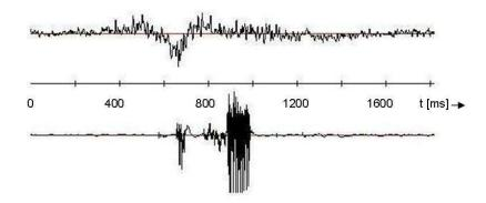
Figure 6.10: EMG and audio signal for the word accept (speaker S0, session 009, EMG1). Muscle activity occurs approximately 200ms prior to sound generation.
