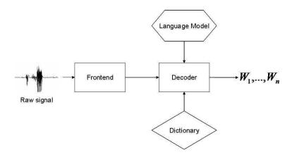
Figure 2.16: Schematic view of a typical speech recognizer
