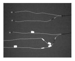
Figure 4.3: Detection electrodes of the VARIOPORT\_III system. Bipolar (upper) and unipolar (lower) electrode configuration.
