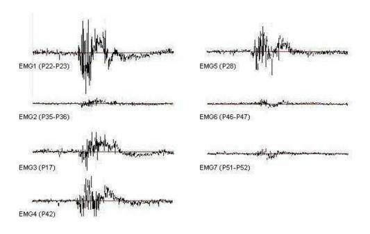
Figure 6.8: Signals for the audibly spoken word zero and electrodes EMG1-EMG7 (speaker S1, session 016).
