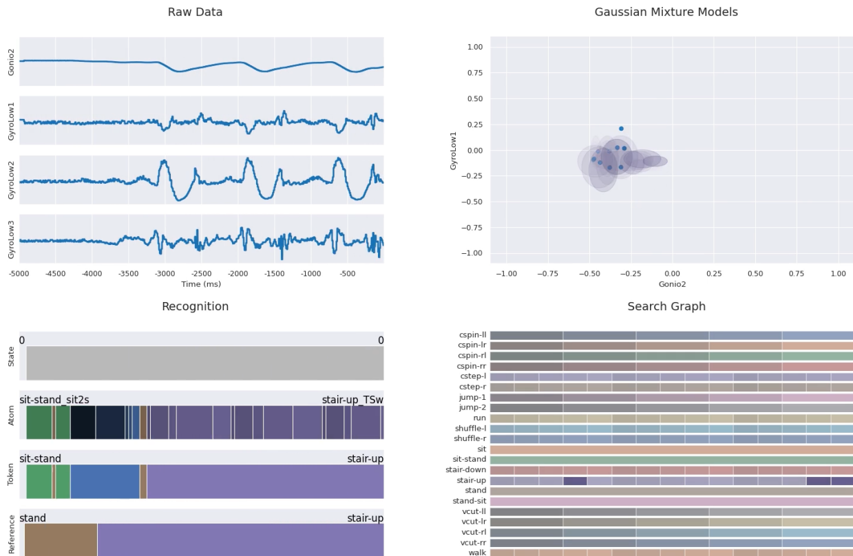
Fig. 1. Online Recognition Mode. The four subplots illustrate the raw data (upper left), the GMMs of the current top three hypotheses (top right), the search graph with the current top three hypotheses (lower right), and the final recognition results (lower left), respectively.
