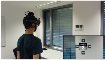
Figure 1: Window blinds control via AR using the SSVEP-BCI paradigm in a room where the menu allows for four operations: blinds up, blinds down, blinds close (fins), blinds open (fins) – the operations are automatically executed via the building’s intelligent control system.
