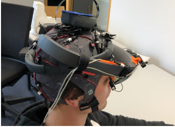
Figure 2: The setup of the EEG cap, the eye tracker, and the HoloLens on the participant
